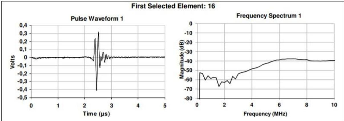
Figure 8 - Pulse waveform (left) and pulse spectrum (right) of a single element of defective L7 transducer
