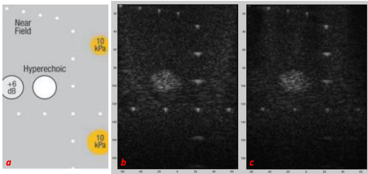
Figure 19 - Captures of the phantom's expected image (a), image from the functional (b) and defective (c) transducers to measure horizontal distance
