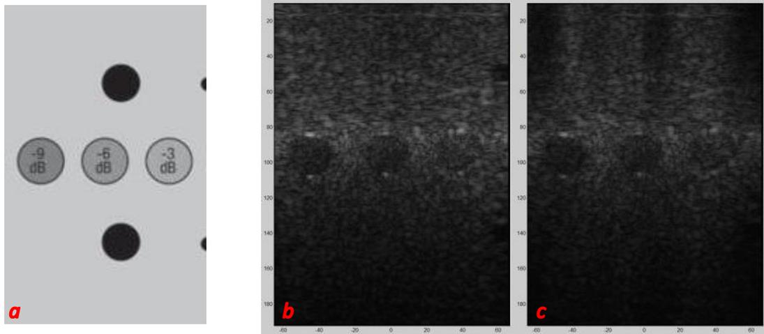
Figure 23 - Captures of the phantom's expected image (a), image from the functional (b) and defective (c) transducers to measure grayscale contrast with the -9dB, -6dB and -3dB contrast targets
