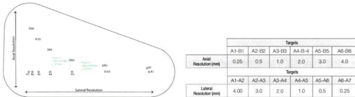
Figure 21 – Combined axial and lateral resolution targets (a) and table listing the distances between them (b)
