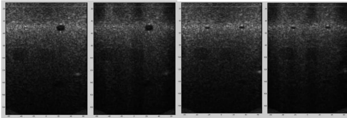
Figure 22- Captures of the phantom image to measure contrast resolution
