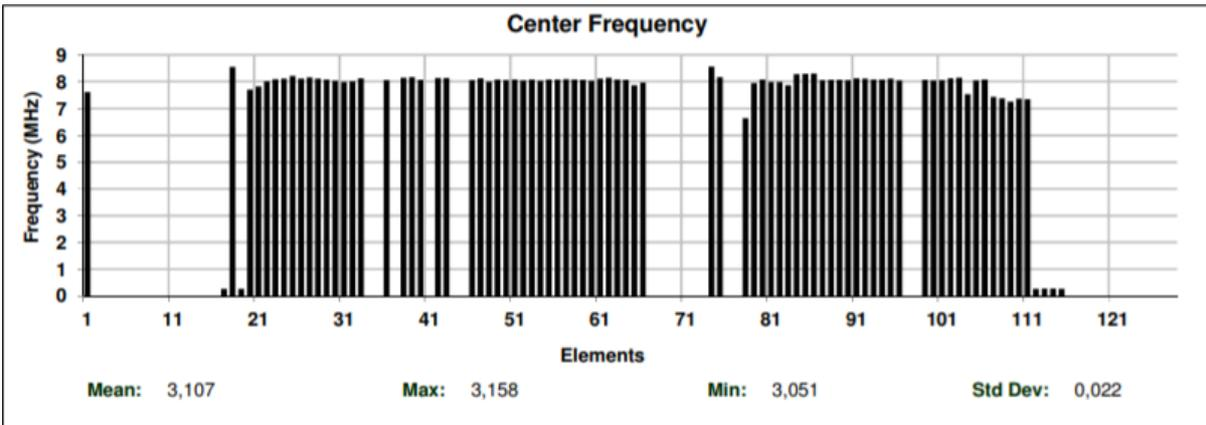
Figure 6 - Center frequency histogram of defective L7 transducer
