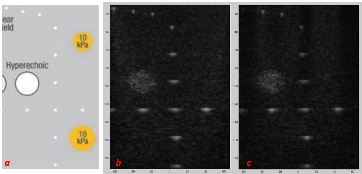
Figure 18 - Captures of the phantom's expected image (a), image from the functional (b) and defective (c) transducers to measure vertical distance
