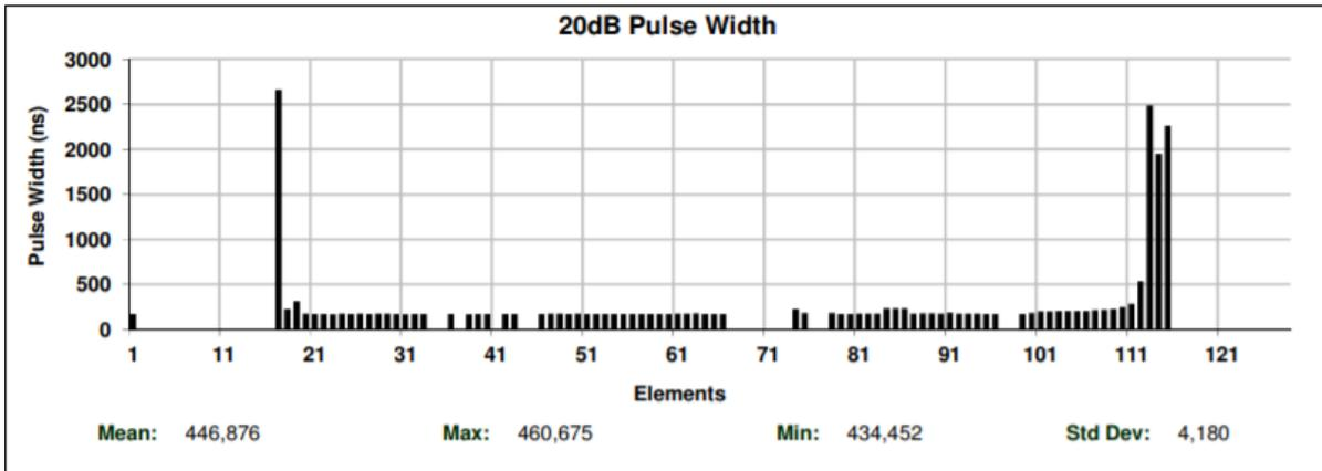
Figure 5 - Pulse width histogram of defective L7 transducer
