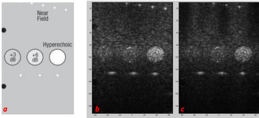
Figure 24 - Captures of the phantom's expected image (a), image from the functional (b) and defective (c) transducers to measure grayscale contrast with the +3dB, +6dB and hyperechoic targets
