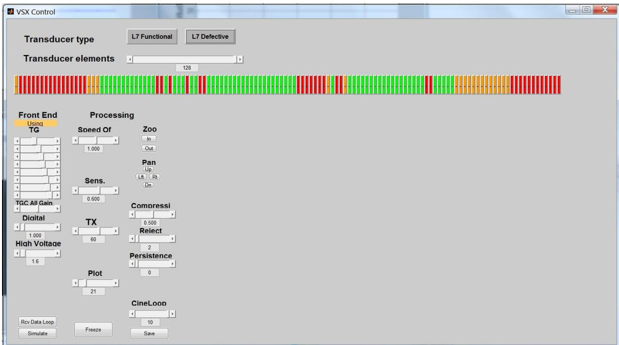
Figure 16 - VSX control window with defective L7 transducer selected
