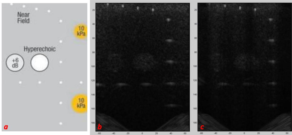
Figure 25 - Captures of the phantom's expected image (a), image from the functional (b) and defective (c) transducers to measure dead zone
