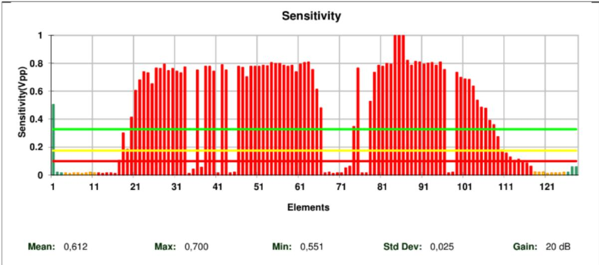
Figure 3 - Sensitivity histogram of defective L7 transducer
