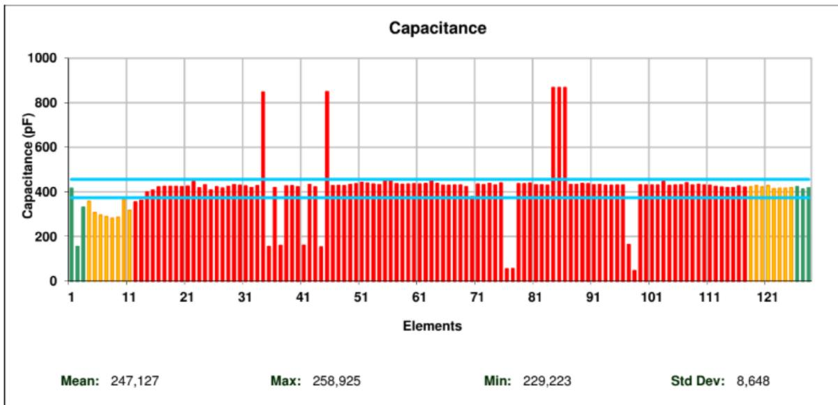
Figure 4 – Total capacitance histogram of defective L7 transducer
