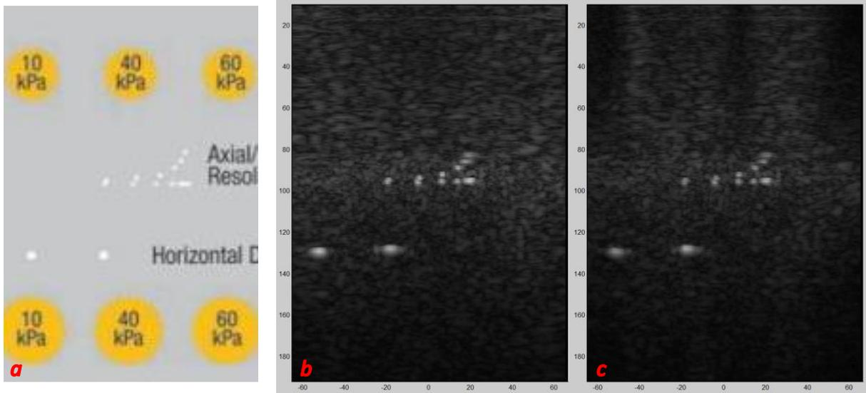
Figure 20 - Captures of the phantom's expected image (a), image from the functional (b) and defective (c) transducers to measure resolutions
