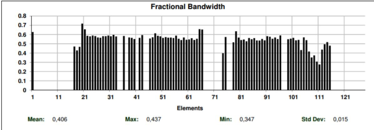
Figure 7 - Fractional bandwidth histogram of defective L7 transducer
