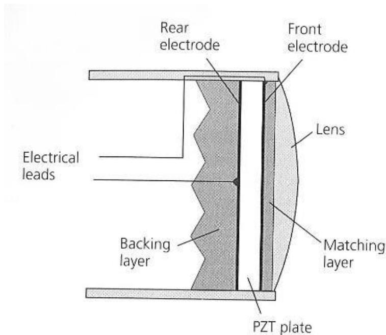
Figure 1 - Main components in a transducer
