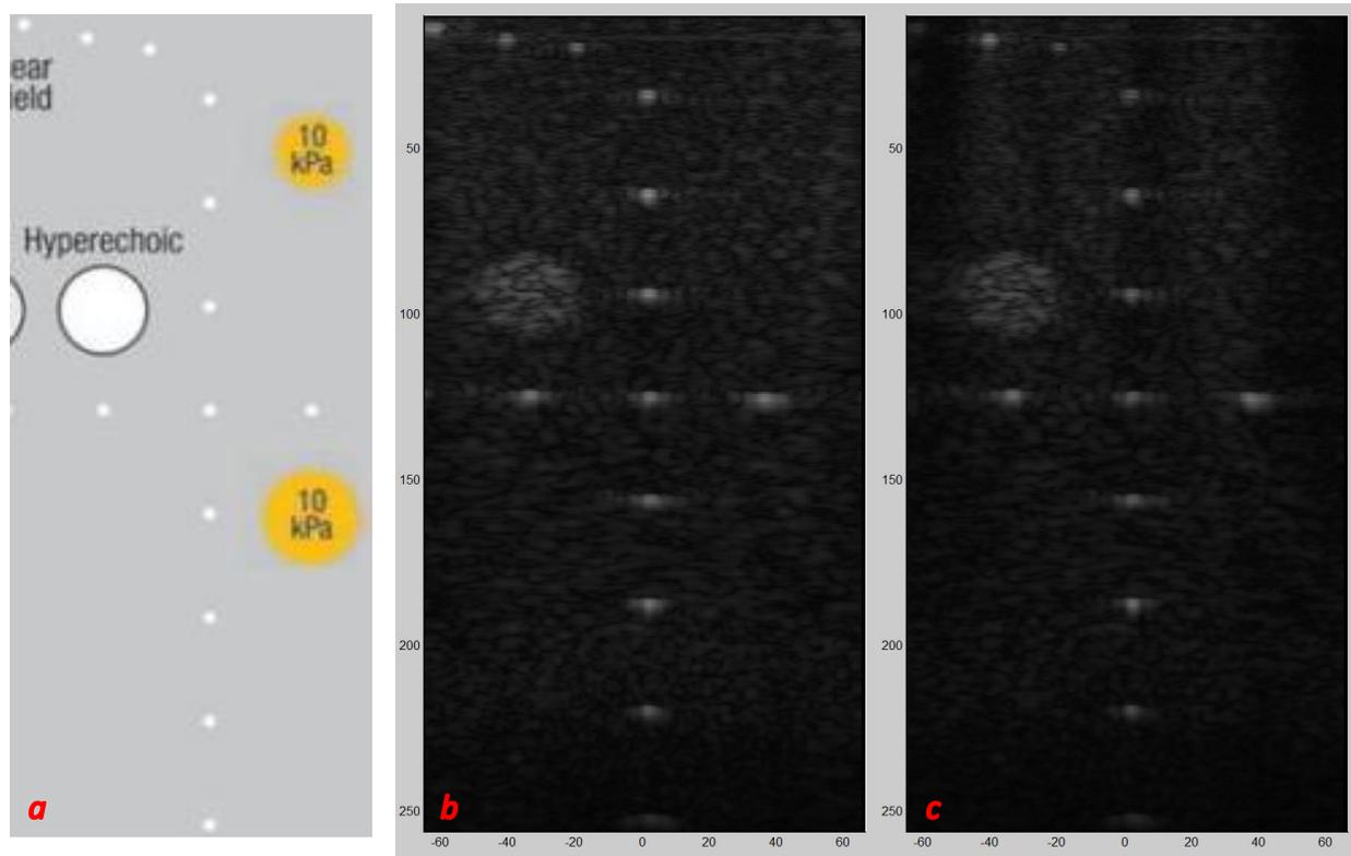
Figure 17 - Captures of the phantom's expected image (a), image from the functional (b) and defective (c) transducers to measure depth of penetration
