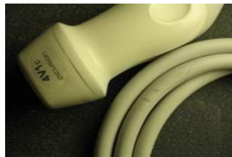
Fig.28 Scratches in the cable
