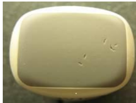
Fig.26 Holes in the lens
