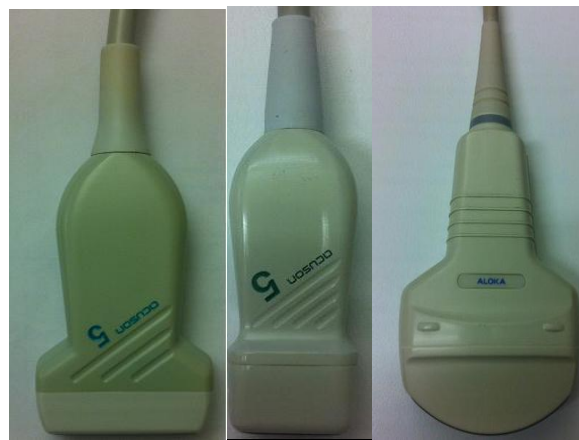
Fig.6 a) Linear array transducer; b) Sector array and c) Curved array
