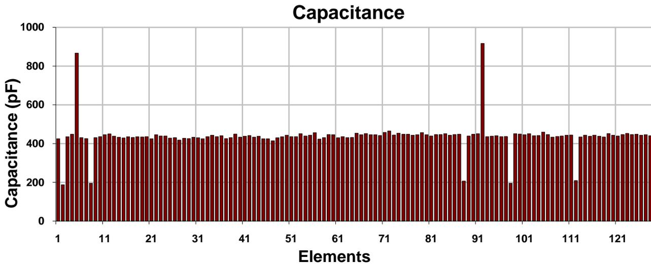
**Figure 9:** The capacitance histogram of a 128 element phased array transducer both with breaks in the cable and short circuits. Break in the cable give capacitance values lower than normal, whilst short circuits give higher. In this transducer there are 5 broken wires and two short circuits. Note that the abnormal values are arbitrary and can assume any value. When it looks like this the wires are broken at the same place.
