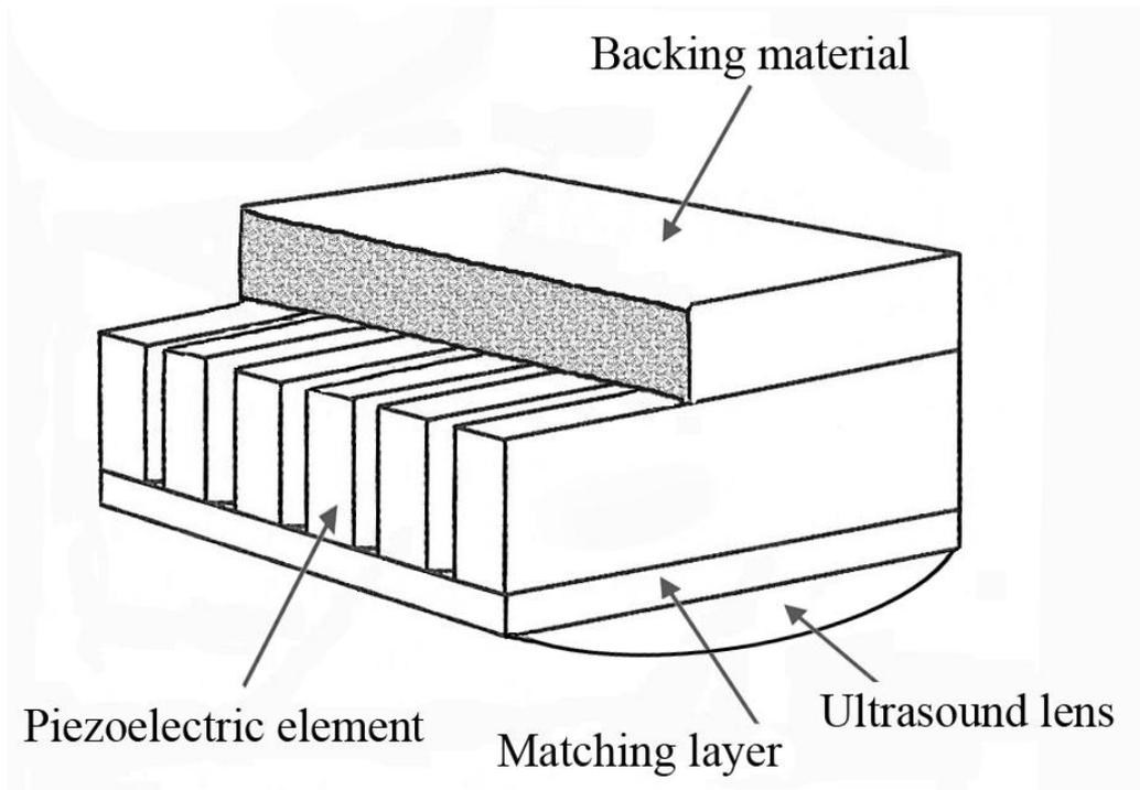
**Figure 3:** The internal parts of an ultrasound transducer.
