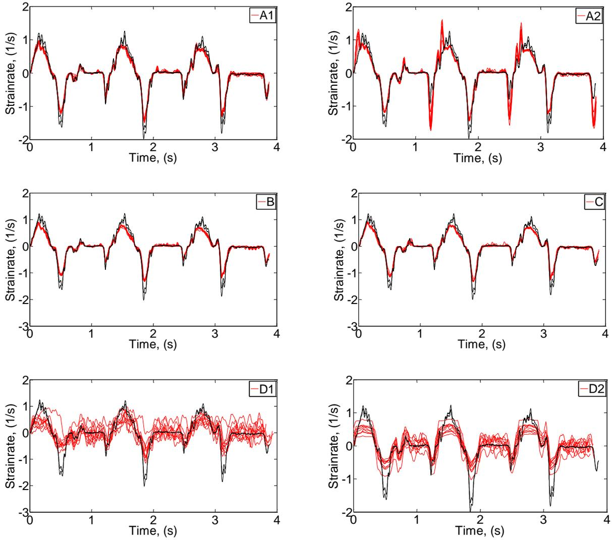
**Figure 25:** The strain rate results of ten repeated measurements by the six ultrasound systems.
