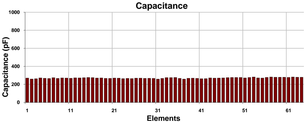
**Figure 7:** The histogram of a 64 element phased array transducer showing the total capacitance (element and wires in both directions) from the Sonora FirstCall Test System.
