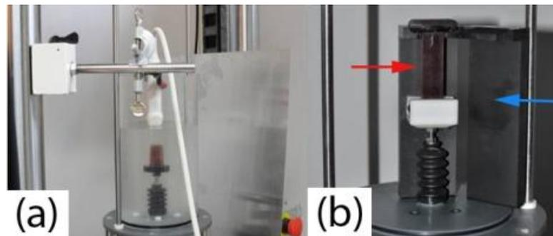
**Figure 13:** (a) Displacement/velocity setup of the phantom. (b) Strain/strain rate setup of the phantom. The water container has been removed and the front part of the suspension device (blue arrow) has been moved and rotated to the right to display the inside of the setup. The tissue mimicking object is shown by the red arrow.
