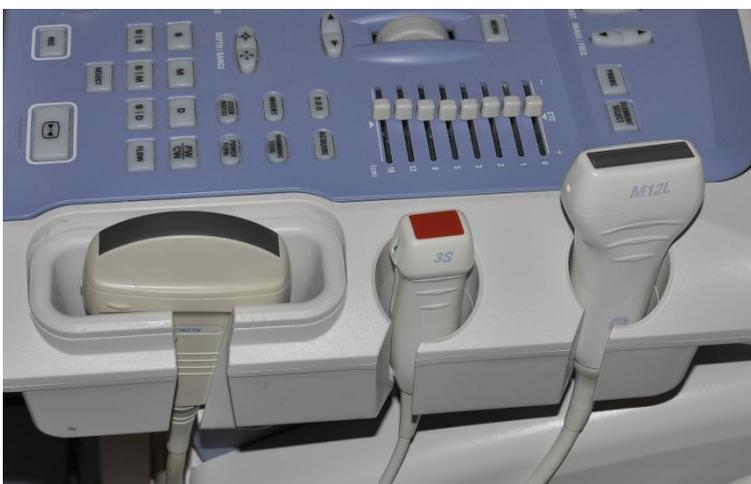
**Figure 4:** Three transducers of different types. The leftmost is a curved linear transducer, the middle is a phased array transducer, and the rightmost is a linear transducer.
