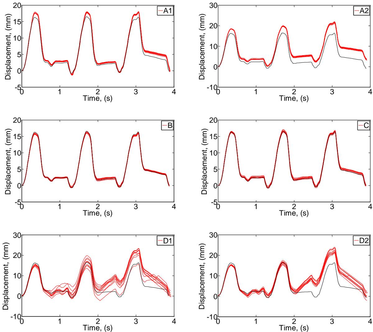
**Figure 22:** The displacement results of ten repeated measurements by the six ultrasound systems
