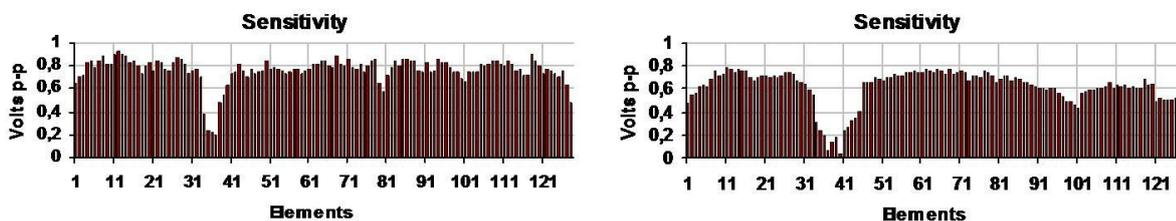
**Figure 19:** Quickly deteriorated transducer. Left panel: The sensitivity histogram of a tested phased array transducer with 128 elements. Right panel: Same ultrasound transducer tested three month later. The peak-to-peak (p-p) amplitude (sensitivity), measures the ability of a transducer to emit and receive ultrasound pulses.
