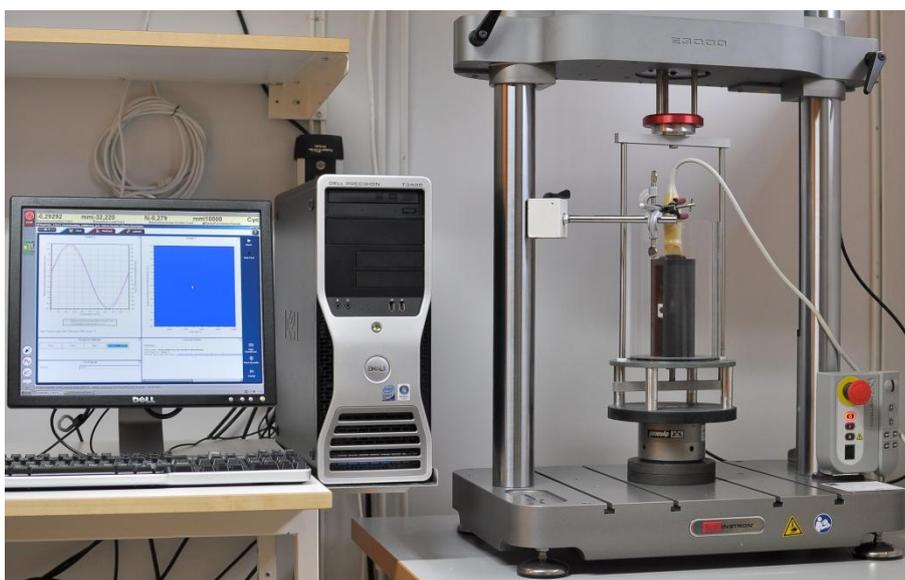
**Figure 12:** The tissue Doppler phantom. Phantom mounted with the strain/strain rate setup.
