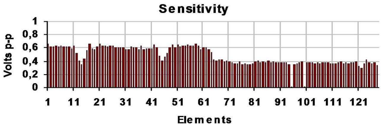
**Figure 21:** New defective transducer. Brand new transducer with two delaminated areas around elements 11 to 17 and 42 to 47, and two broken signal wires affecting element 95 and 100. The peak-to-peak (p-p) amplitude (sensitivity), measures the ability of a transducer to emit and receive ultrasound pulses. This transducer is designed with elements having two sensitivity levels for increased focusing properties.
