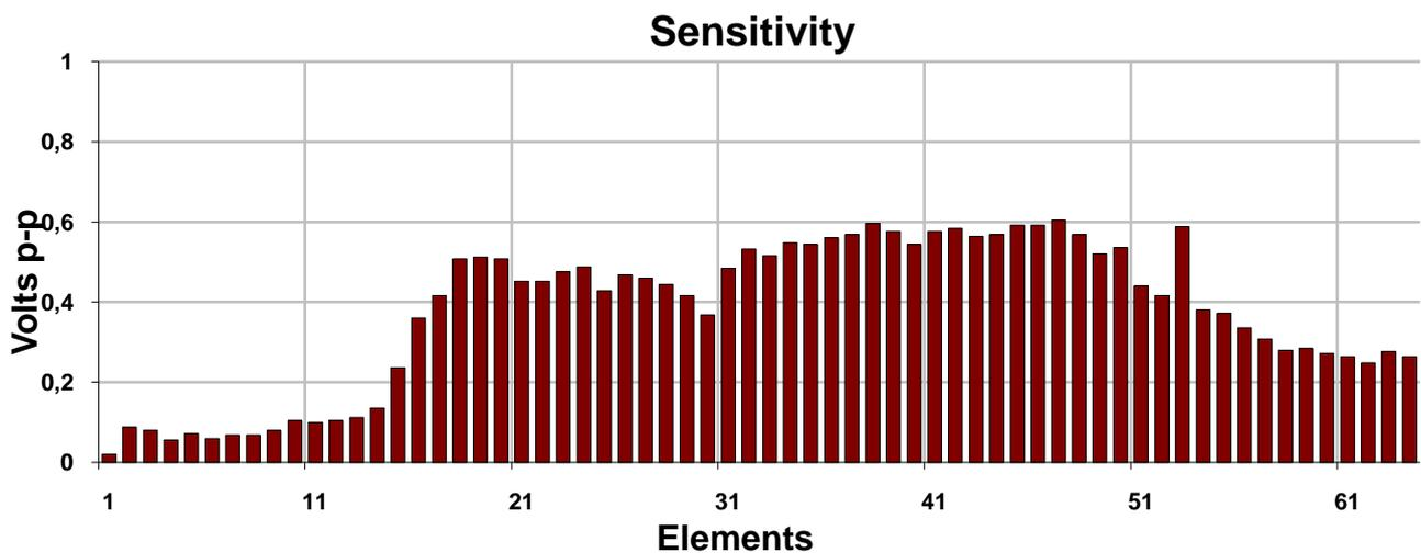
**Figure 8:** The sensitivity histogram of a delaminated 64 element phased array transducer. Note that 0.6 is the expected value and how differently the elements are affected. The peak-to-peak (p-p) amplitude (sensitivity), measures the ability of a transducer to emit and receive ultrasound pulses.
