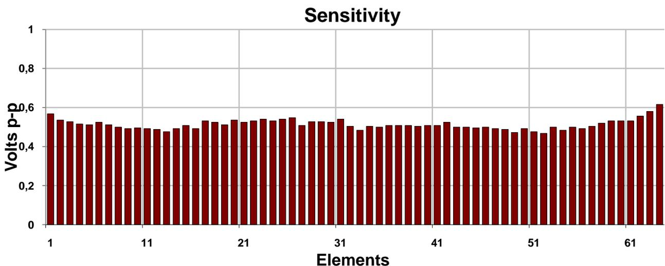
**Figure 6:** The element sensitivity histogram of a 64 element phased array transducer from the Sonora FirstCall Test System. The peak-to-peak (p-p) amplitude (sensitivity), measures the ability of a transducer to emit and receive ultrasound pulses.
