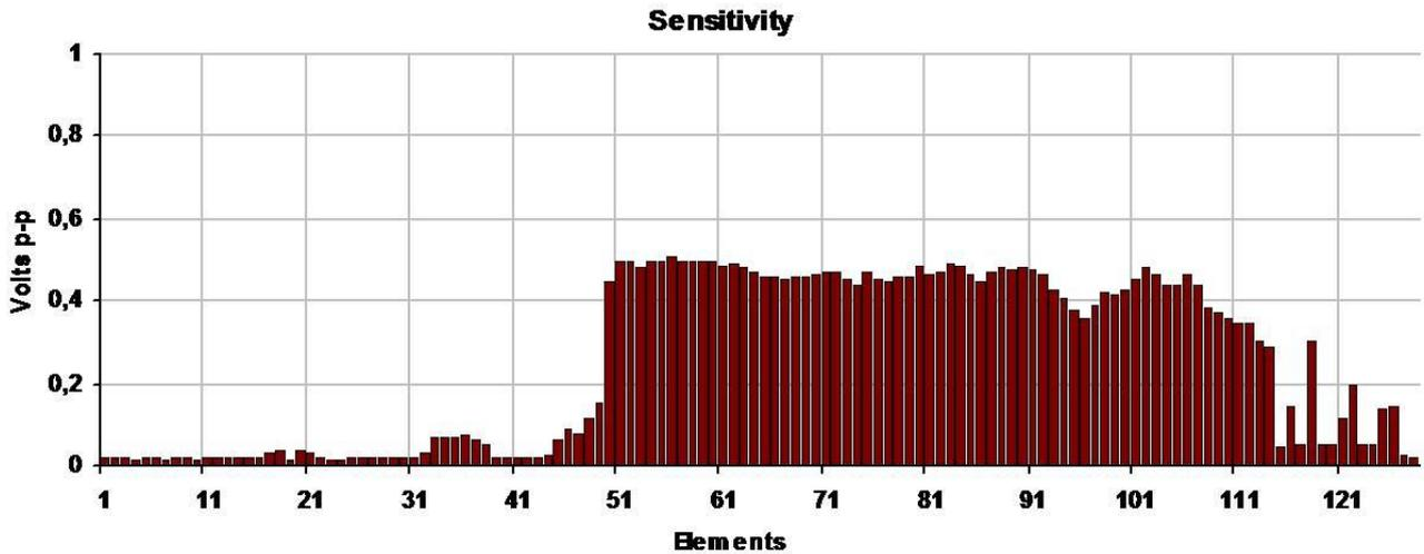
**Figure 20:** Defective transducer not realized by the user. Defective transducer found at the department of radiology at Karolinska University Hospital. The peak-to-peak (p-p) amplitude (sensitivity), measures the ability of a transducer to emit and receive ultrasound pulses.
