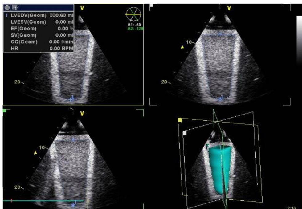
**Figure 5:** One of the volume phantoms in Study I imaged by the tri-plane method, a simplified 3-D ultrasound imaging technique. 3-D; three-dimensional.
